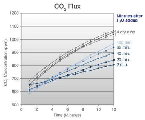
**Simulated rain event in closed-system chamber lab study:** Concentration time series for dry and wet dirt measurements of N<sub>2</sub>O, CH<sub>4</sub> and CO<sub>2</sub> are shown. After adding water, N<sub>2</sub>O emission rate triples in 2 min and continues to rise, while CH<sub>4</sub> emission rate spikes and then decreases, and CO<sub>2</sub> emission rate is suppressed but recovers slowly. Contact Picarro for more details and the latest data related to this study.
