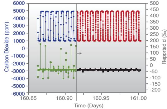
*Fast concentration fluctuations can cause unwanted systematic errors in the reported  $\delta^{13}\text{C}$  isotope ratio from CO<sub>2</sub>. Picarro's G2101-i instrument has a faster measurement rate and an algorithm designed to minimize cross-talk between <sup>12</sup>CO<sub>2</sub> and <sup>13</sup>CO<sub>2</sub> spectral features, thereby producing high quality data, even under challenging conditions of rapidly changing CO<sub>2</sub> concentration.*
